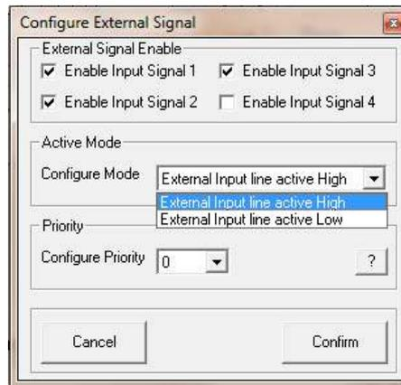
Furthermore, it is also possible, in case more Events related to the Input Switches are occurring at the same time, so activating at the same time more than one Switch, to assign a Priority in "serving" the events related to the active Switches (see below).
