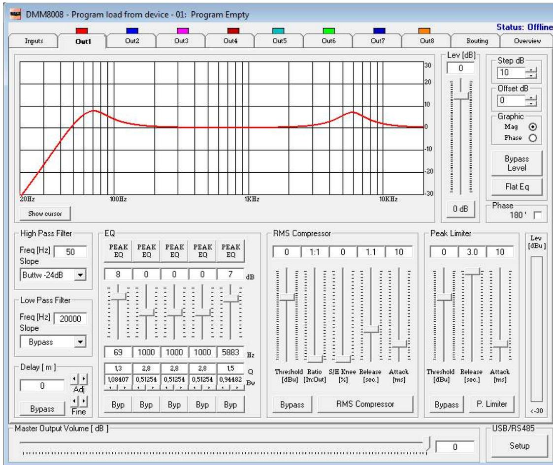
**High Pass Filter:** from this sub-frame it is possible to set the Output Channels High Pass Filter (HPF).
