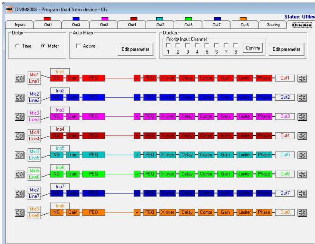
Within the Overview Page, can be checked the all channels inputs selection (between Microphone and Line), so as any of the available processes can be accessed double clicking on its name in the processes' block diagram. Particularly, in this page is also resumed the current selections operated for the Inputs in terms of available Eq or Feedback Eliminator processes, when Microphone Input is selected.
