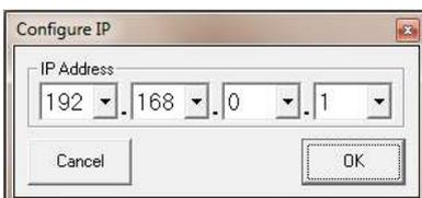
Enter the IP address of the unit desired and then press "OK" to confirm. For each unit, a separate window is added.
