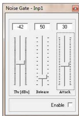
**Gating Threshold:** the gating threshold is ranging from -80dB up to 0dBu.
