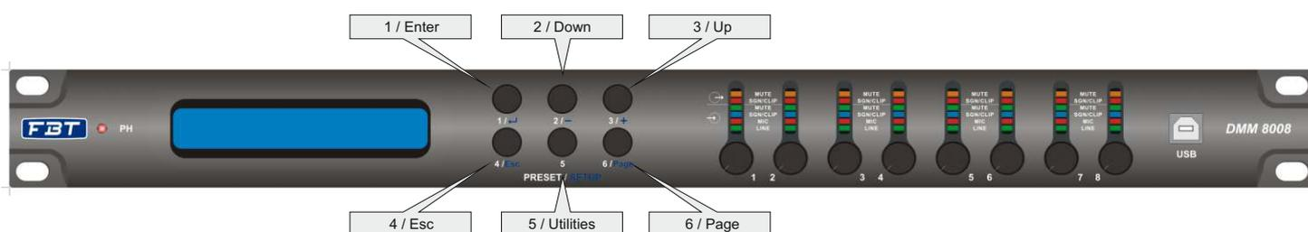
Referring to the Picture, in order to access the System Setup need to press the Button 5 / Utilities, for about 4 seconds, The following window will appear:
