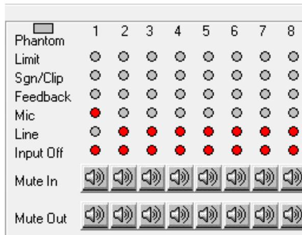
The line of "Input Off" leds is indicating when an Input is Off or Muted by the Noise Gate.
