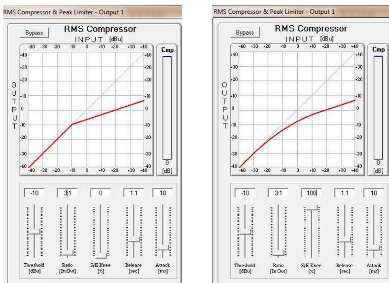
**"Threshold"**: the selectable range of the RMS Compressor's Threshold is from +14,2dBu (OFF) to -33,8dBu in steps of 0.2dBu
