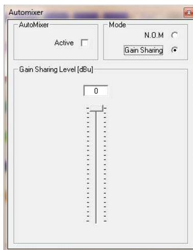
If selected the Gain Sharing option, the Max Gain available to the SUM of the all microphones can even be set using the Gain Sharing level Slider.
