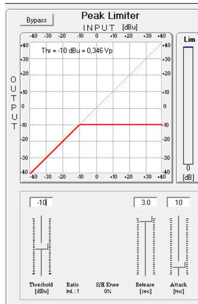
“**Threshold**” : the selectable range of the Peak Limiter's Threshold is from +14,2dB (Limiter not active) to -33,8dB in steps of 0.2 dB.
