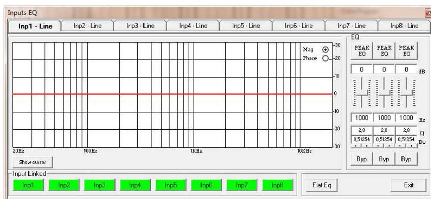
**EQ:** from this sub-frame it is possible to set the Input Channels three available Peaker (Bell) or variable Q Shelving Filters.
