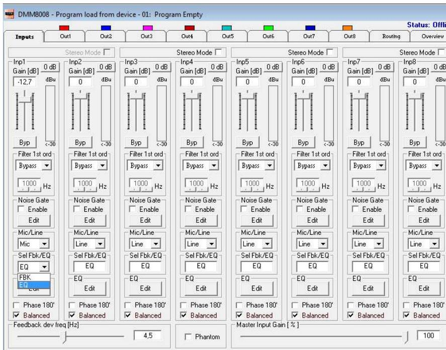
When selected microphone as input, the user can chose to select on the input itself a 3bands Eq process on the Input signal, or a Feedback Eliminator.
