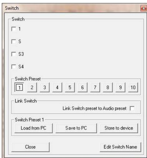
The switches controlled by this window actually set as 0V or 5V the physical 4 output "switch" lines available on the DMM 8008 back panel and useful for controlling remote devices.
