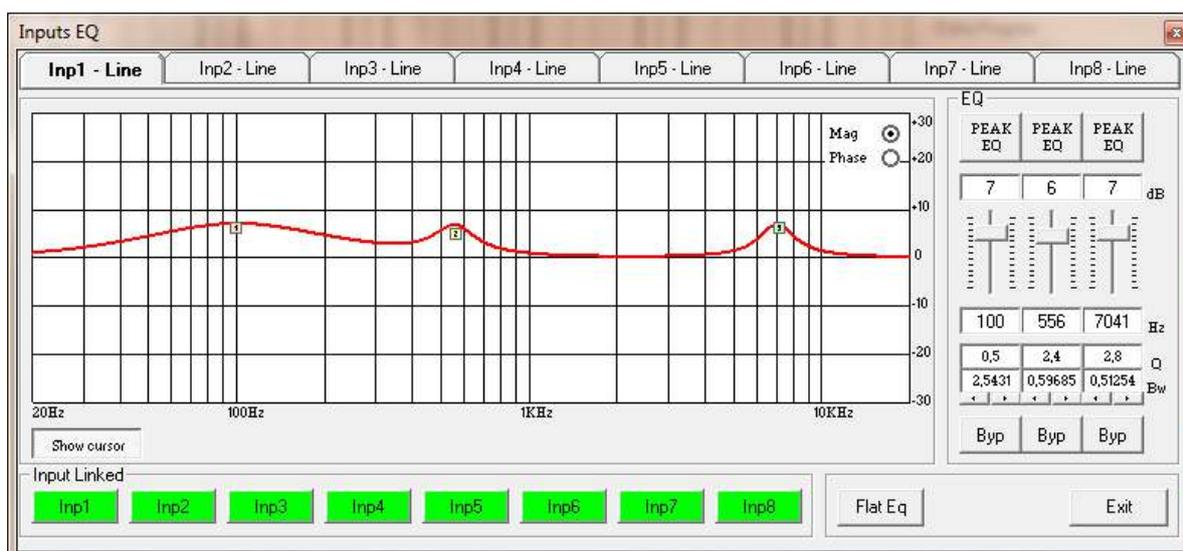
Once the all 3 available cursor are shown on the Frequency Response graphic, just selecting anyone of them with the mouse's arrow and maintaining the mouse's click pressed, it is possible to move and place the selected cursor on the desired frequency and with the desired gain.
