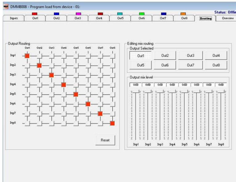
The routing Page is allowing to set the Matrix Structure of the DMM 8008 and to assign to each Output the desired Inputs.
