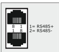
The output jack RS485 OUT (12) may be connected to the jack RS485 IN of an additional DMM 8008. Thus, up to 64 units to be controlled may be connected in a chain. If multiple units are connected and if longer control lines are used, the control output of the last unit in the chain should be equipped with a terminal resistor (120 Ohm resistor between pin 1 and pin 2 of the connection) to prevent interference while signals are transmitted.
