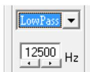
Once active, the smooth first order LP filter is intended to be mainly used with the microphone's input selected, in order to reduce the amount of high frequencies without affecting significantly the voice quality, nevertheless increasing the immunity to the Feedback.
