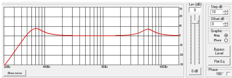
Once the all 5 available cursor are shown on the Frequency Response graphic, just selecting anyone of them with the mouse's arrow and maintaining the mouse's click pressed, it is possible to move and place the selected cursor on the desired frequency and with the desired gain. For setting the filter's Q, still need to enter the desired value directly in the dedicated box in the filters' editing main sub-frame.
