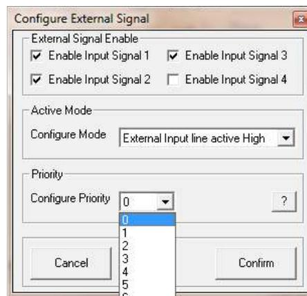
The desired Priority can be set selecting one of the 8 options available, corresponding to the following Priority Table (accessible pressing the "?" button aside the "Configure Priority" selection box):
