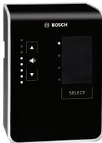
The wall control panel is used to select the input source and to adjust the audio volume level in the pre-selected loudspeaker zones. The wall control panel uses the same CAT-5 cabling as the PLM-8CS 8 Zone Call Station with communication via RS485 and is also powered from the PLM-8M8 DSP Matrix Mixer. The supplied wall-mount bracket is used to install the wall control panel.
