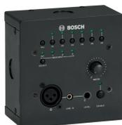
The PLN-4S6Z Wall Panel is used to remotely control the All-in-One Unit. It is connected to the All-in-One Unit using a Cat-5 cable terminated with RJ45 connectors.
