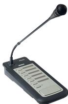
The PLN-6CS Call Station is a remote device for making announcements to selected zones of the All-in-One System. A maximum of six Call Stations can be connected in a daisy chain configuration to the All-in-One Unit using Cat-5 cables terminated with RJ45 connectors.
