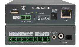
TERRA-IEX is a 2 channel audio over IP encoder/decoder.
