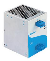
The PRA-PSM24 power supply module is a compact DIN-rail mounted power supply, delivering 24 V at up to 10 A continuously. This power supply is an OEM power supply, made for Bosch by Delta Power Supply, as a cost effective alternative to the PRAESENSA multifunction power supply PRA-MPS3 to power a PRAESENSA system controller or other devices and utilities that need 24 V, in case the additional functions and characteristics of the multifunction power supply are not needed.
