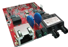
NET2-SR RJ45(B)-Fiber Single(A)
