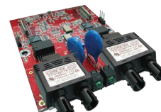
NET2-SS Fiber Single(B)-Fiber Single(A)
