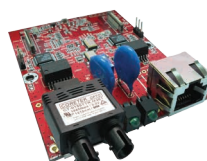
NET2-RM Fiber Multi(B)-RJ45(A)
